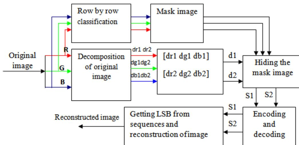
Fig. 1. The Flow of Proposed Algorithm on Color Images
